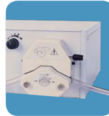
Sterile Tubing P/N 2521-0219 Enables aspiration and retrieval of tissue
